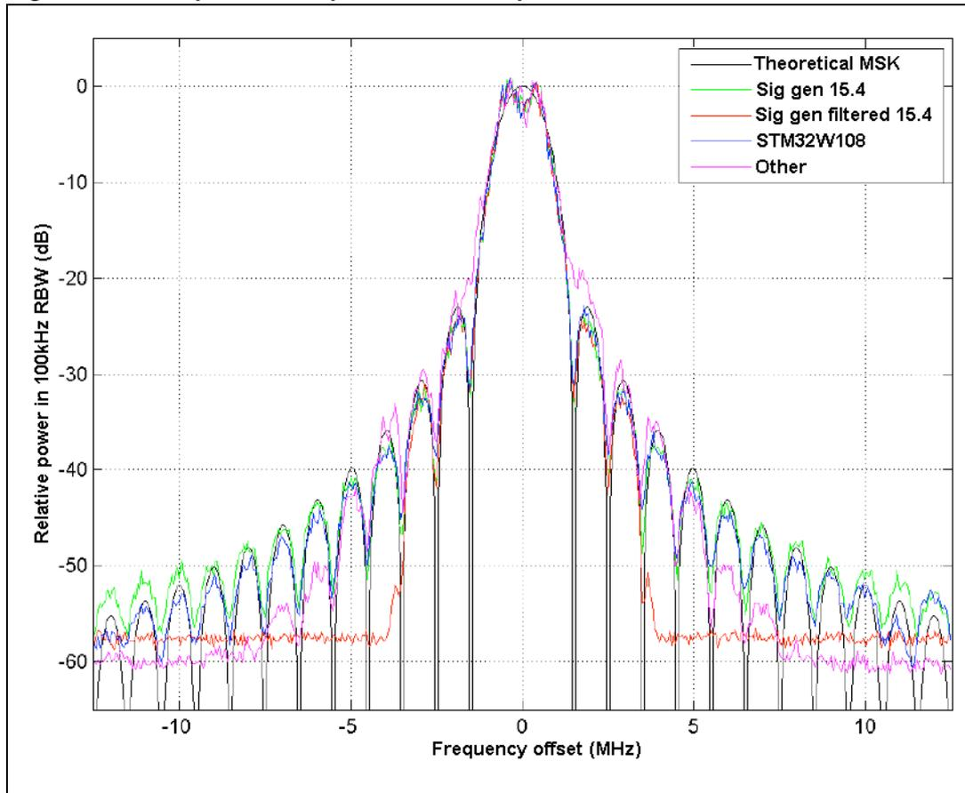
It can be seen that the heavily filtered 15.4 signal generated by the signal generator is not representative of either type of modulation technique, and therefore does not give a useful measure of real performance.
