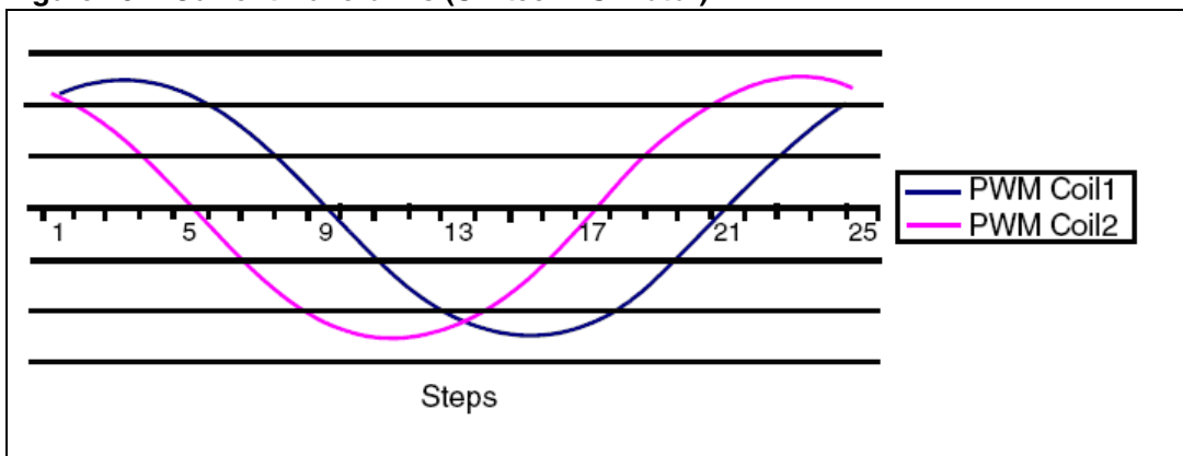
Figure 10. Current waveforms (Switec M-S motor)
